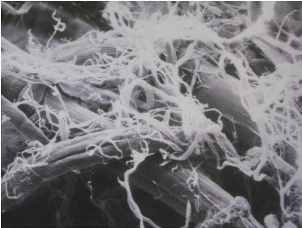
***SEM Photomicrograph - CFF Fibrillated Fiber***
